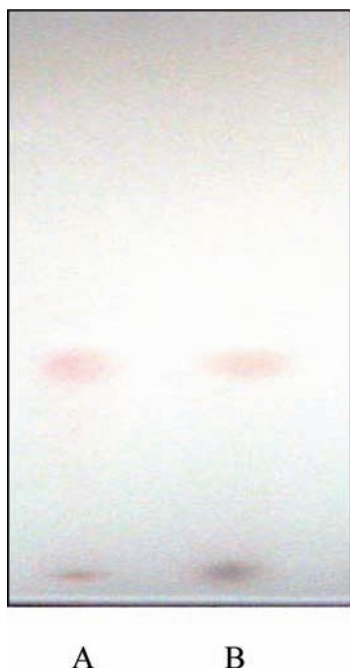
Figure 2. TLC of the (A) standard Me-Cbl and (B) HPLC fraction of Me-Cbl from the S. platensis sample.
